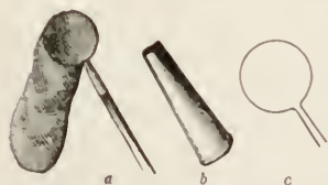
FIG. 44.— a , net; b , ferrule to receive handle; c , wire hoop to be fastened in the upper end of the ferrule (Riley).
